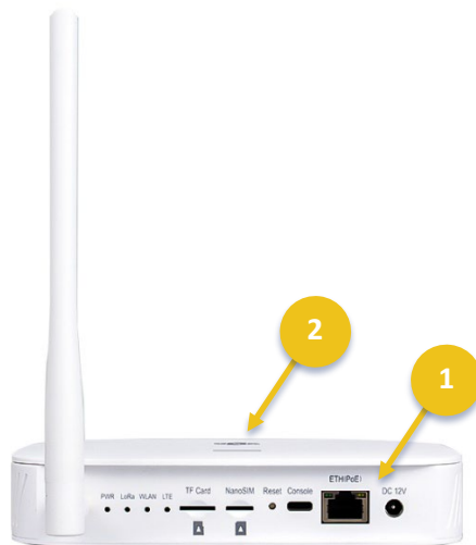
Figure 5 – Plug AC power cable into DC 12V input
