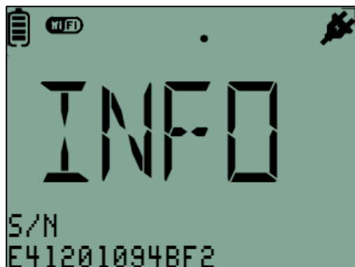
Figure 32 – Use the right and left arrows to scroll through logger information
