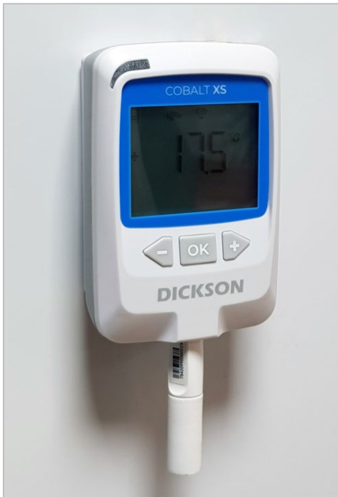
Figure 8 – Placing Cobalt XS Wi-Fi on a metallic surface with magnetic mount
